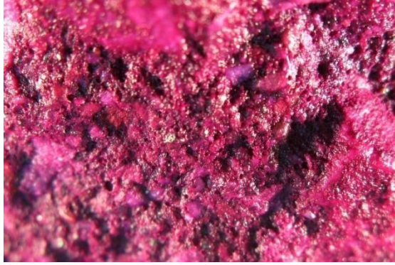
Specimen Prepared with Air Entrainment
